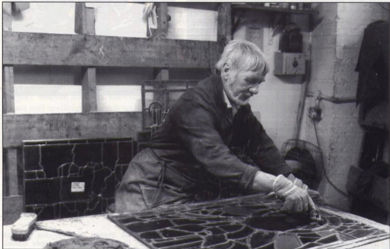
Cement putty is forced into the lead.
